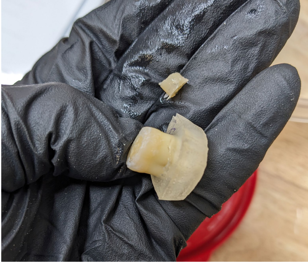
Figure 3. Failure mode 2 (clean breakage)
