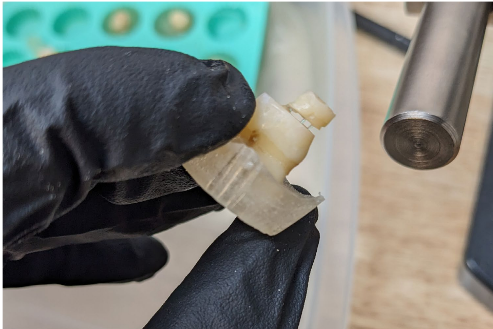
Figure 2. Failure mode 1 (slight separation)
