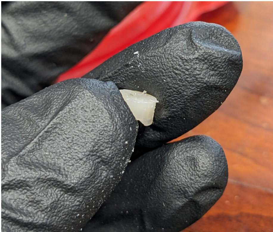
Figure 5. Pins shearing in group 2 samples when there was a clean break
